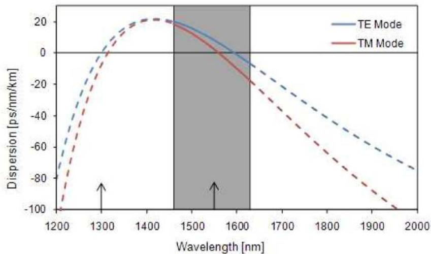
Fig. 2. Dispersion curves for the quasi-TE and quasi-TM modes. The shaded region indicates the experimentally measured wavelength range (solid lines); the dispersion is extrapolated outside this region (dashed lines). The two input pulse wavelengths are illustrated by the vertical arrows.
