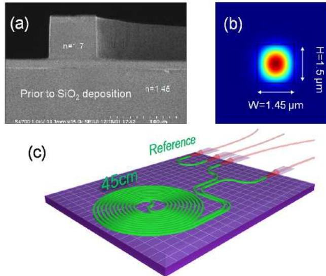
Fig. 1. (a) Scanning electron microscopy image of the cross-section of the high-index waveguide prior to the final deposition of the SiO<sub>2</sub> upper cladding. (b) Theoretical mode profile and (c) Top-down schematic view of the 45cm long spiral waveguide.
