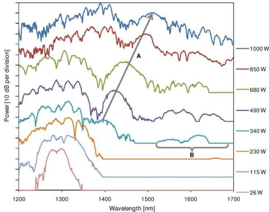
Fig. 4. Experimental output spectra for different input peak powers at 1288 nm. The offset between spectra is proportional to the peak power. (A) and (B) are features described in the text.
