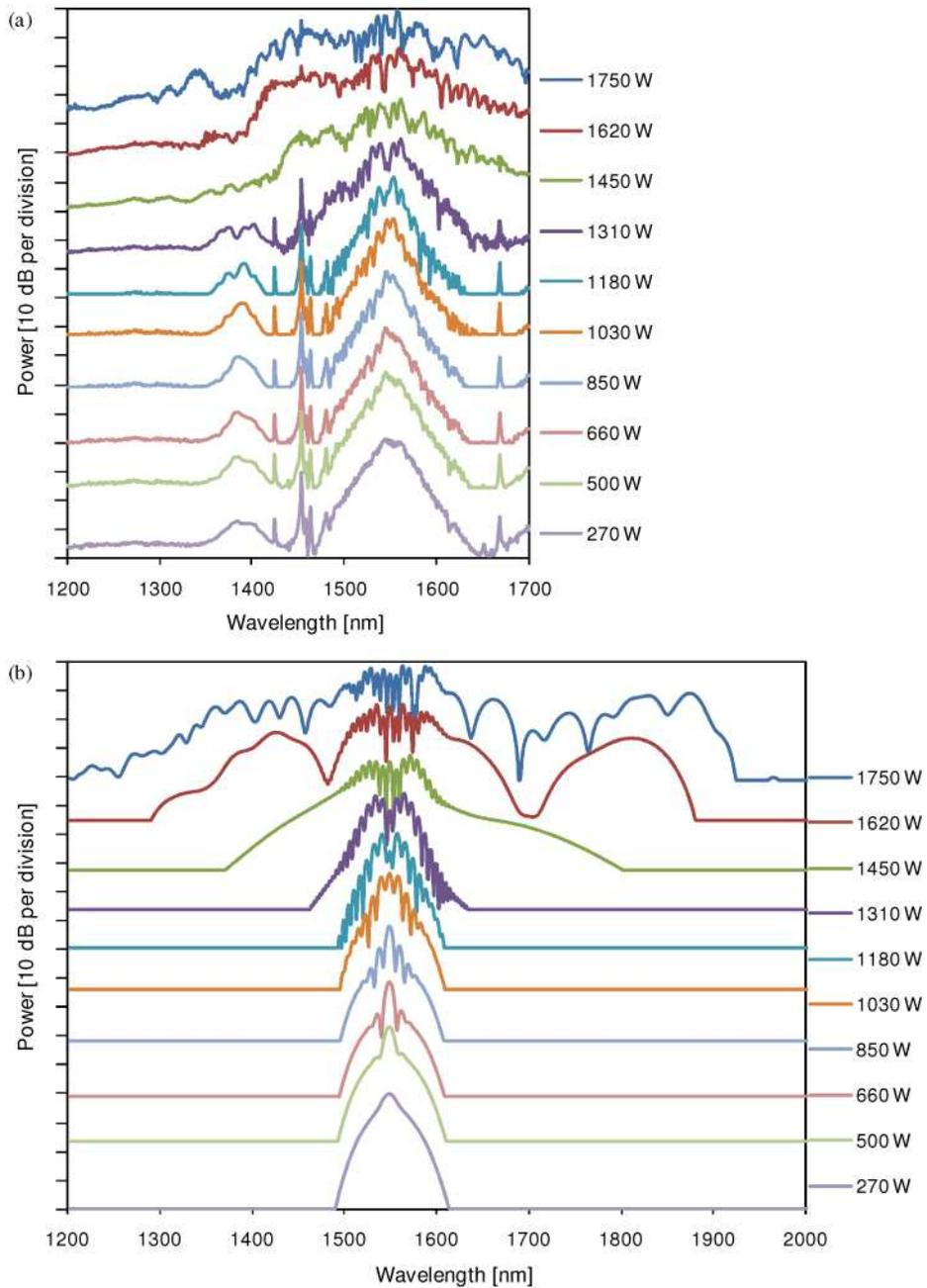
Fig. 3. (a) Experimental and (b) simulated output spectra as a function of coupled peak power for optical pump pulses at 1550 nm. The offset between spectra is proportional to the peak power.
